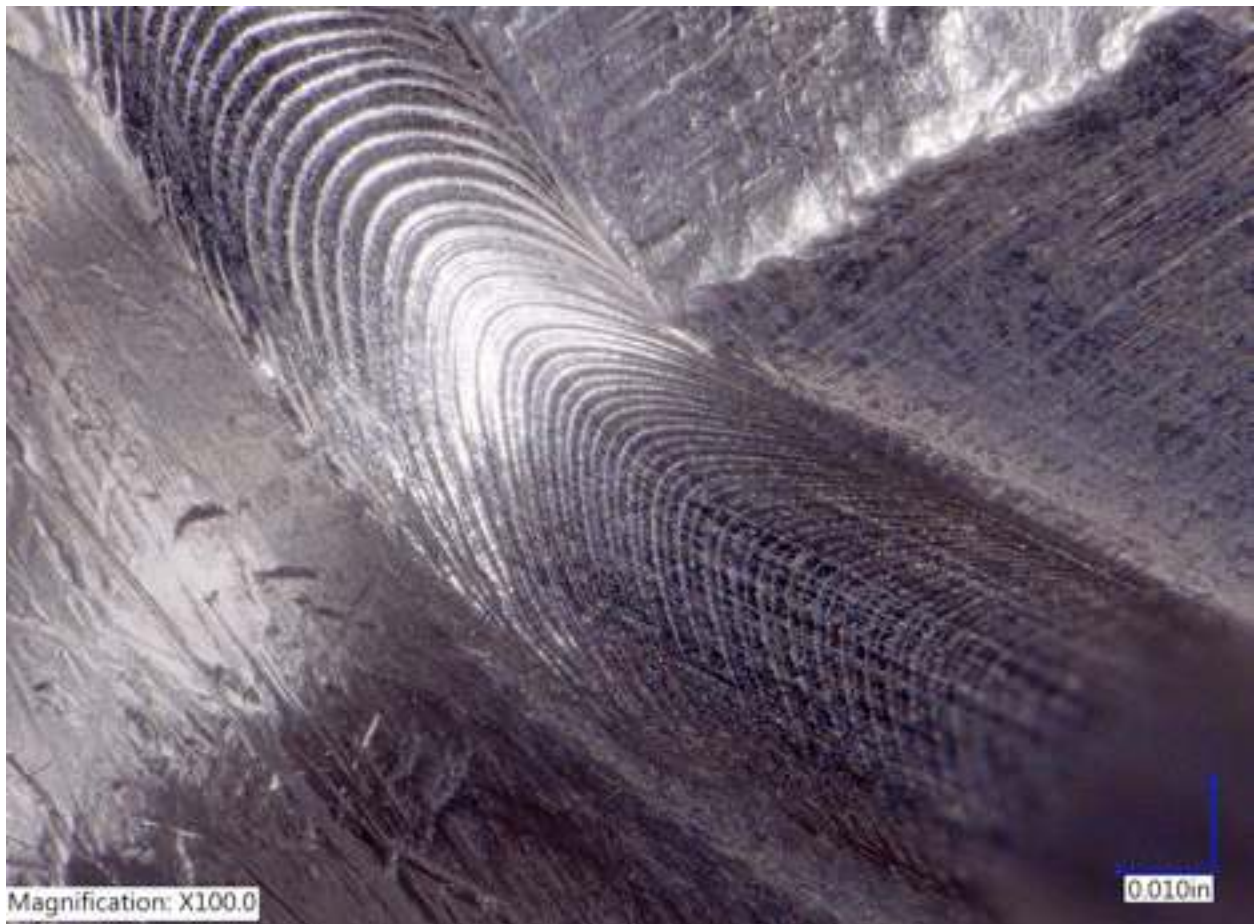
A laser weld in stainless steel
